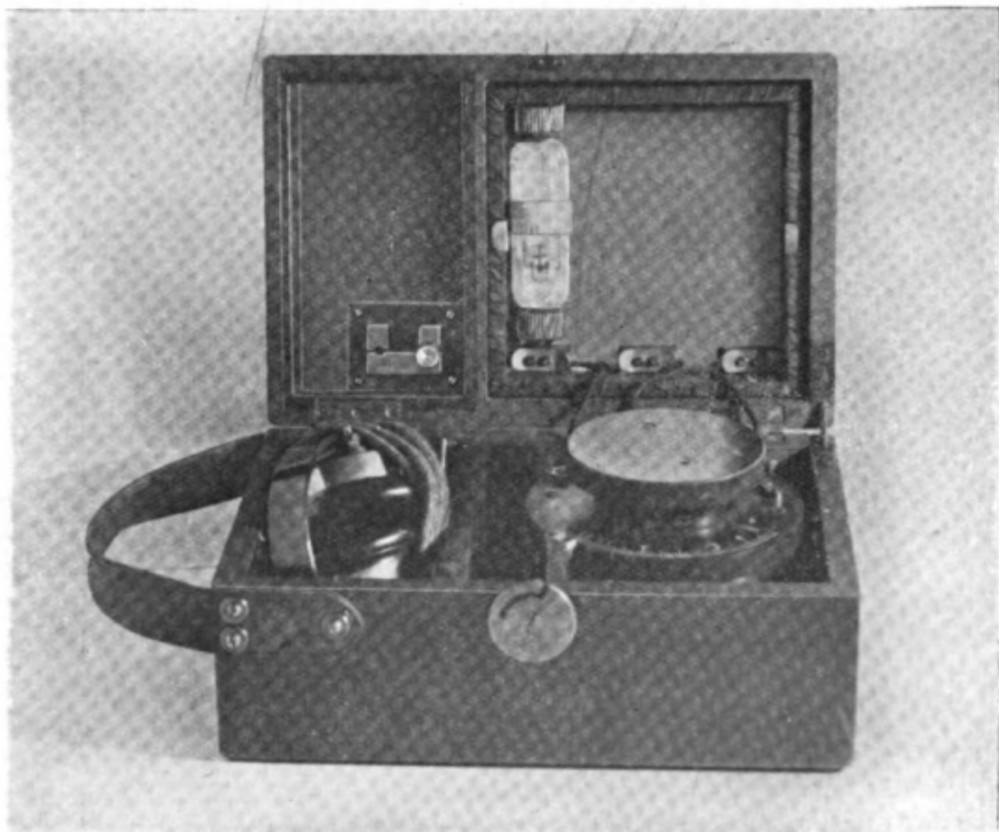
THE MARCONI VACUUM AMPERE GAUGE MOUNTED IN A WAVE-METER.
